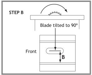
Figure 94. Making the second slot-to-blade measurement at 90°.
